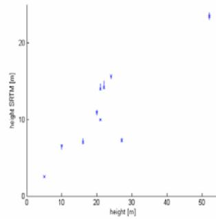
Fig. 7: Tell heights of the SRTM model tend to underestimate the real base-to-top height of the mound (from topographic maps) systematically.
