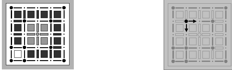
Fig. 7. left: a block complex (cf. figure 2 right); right: possible positions of the block complex \sigma -circulator around the black 0-cell – only two 1-cells (black) belong to a 1-block, the other two (gray) are ignored because they belong to a 2-block
