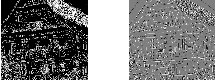
Figure 3: Left: Edges obtained as zero crossings of the appropriate scale image (detail). Right: Nonmaxima suppression of appropriate scale ridges (black: maxima, white: minima) (detail)
